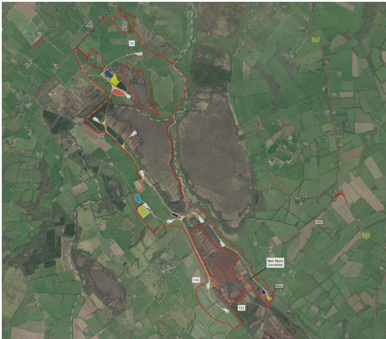
Fig. 13: Proposed Turbine Layout in the Context of Birr and Surrounding Receiving Environment (Source: Applicant Drawings)
